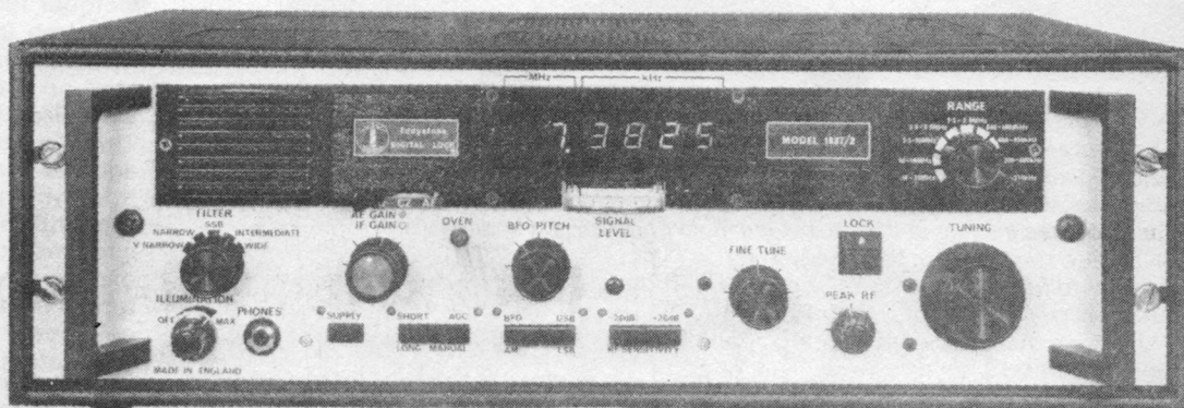
Introduced in 1979, the 1837/2 communications receiver which covered from LF to 30MHz
