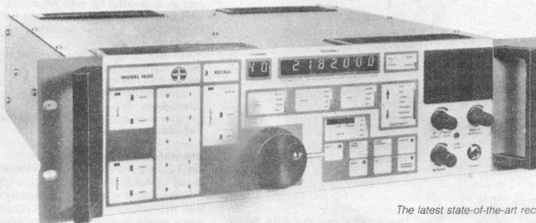
Introduced in 1979, the 1837/2 communications receiver which covered from LF to 30MHz
